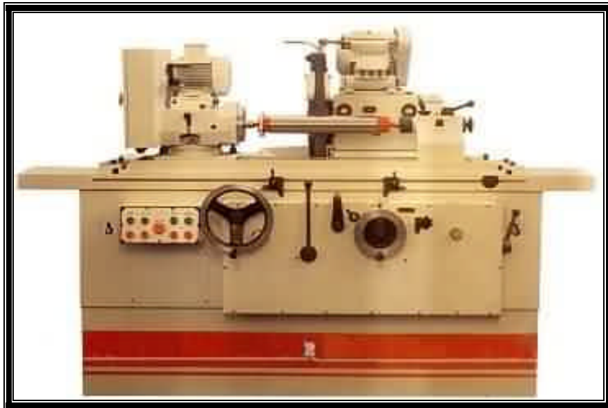
Picture 2. 24: The Grinding Machine for Grinding Cylindrical Surfaces
