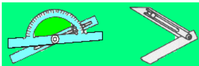
Figure 2.15: Types of angle protractors
