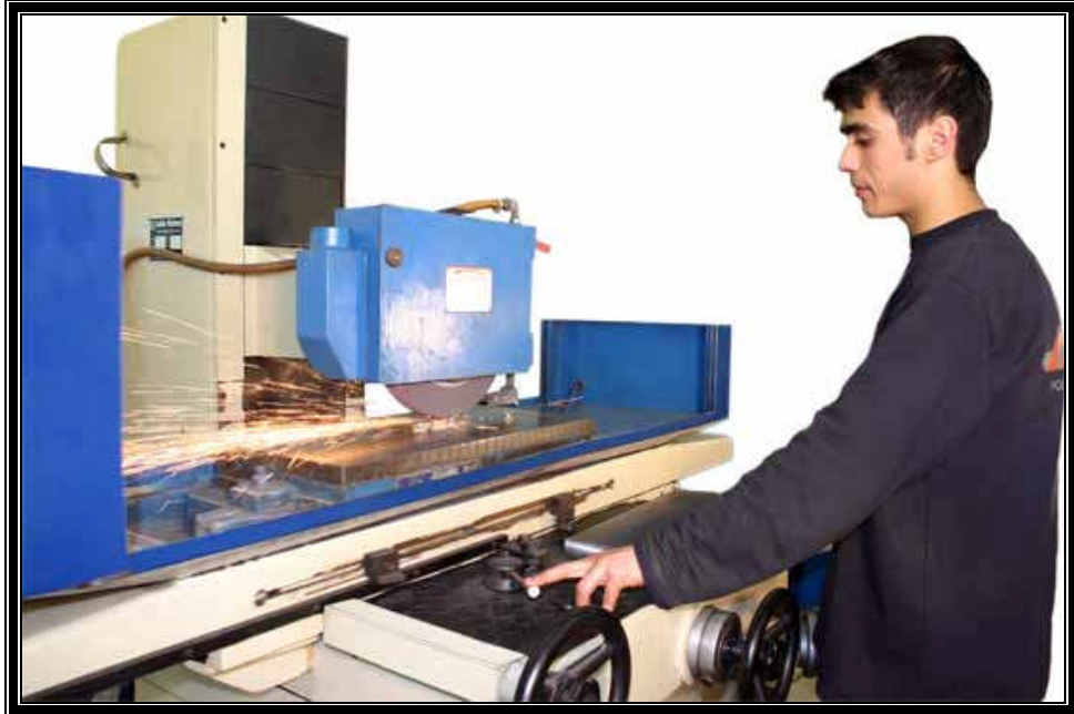
Picture 2. 23: Grinding The Flat Surfaces With A Surface Grinding Machine
